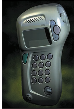
Figure 1.44 A computer-rendered image created by the technical illustrator using the CAD model
